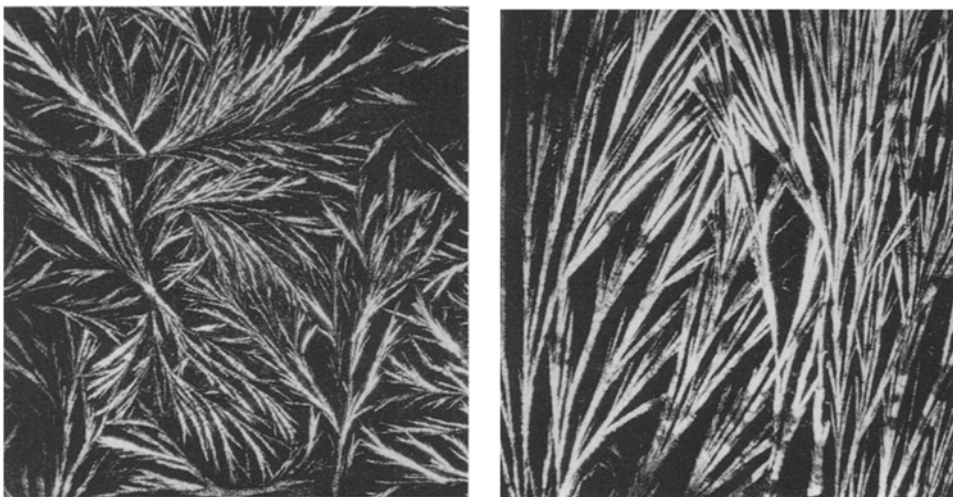
Fig.1 Photomicrographs of different forms of assymetrical sheaf-like crystalline forms of the PDXO-Fe(III) chloride (7:3) complex observed after 30 seconds exposure to pyrrole vapour. Scale bar 50 \mu m.
